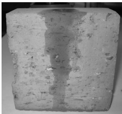
Fig. 1 Ceramic brick filled by siloxane injection
