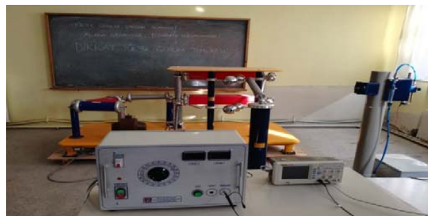
Fig. 7 200 kV lightning impulse voltage generator and water jet test system
