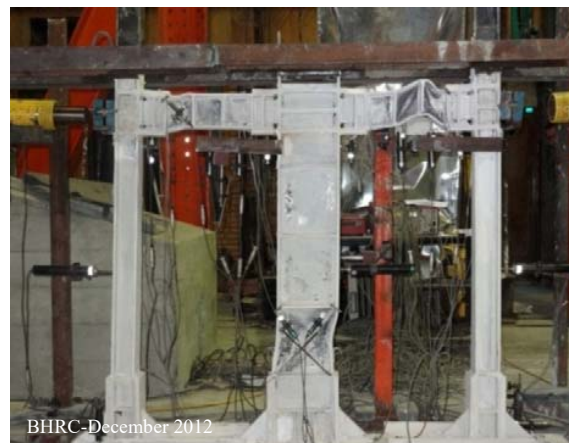
Fig. 6 TRF frame deformations at the last cycle of experiment (33rd)
