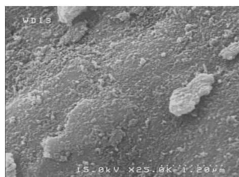
Fig. 12 The FE-SEM image of Al-MWCNT after the mixing process
