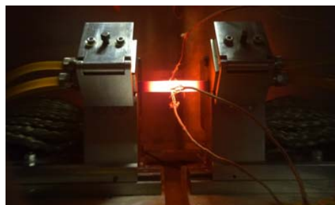
Fig. 2 Sample with thermocouples during heating
