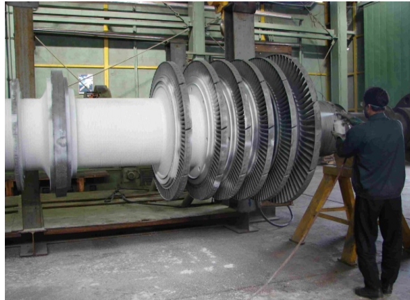
Fig. 3 Spraying calcium carbonate solution over the rotor surface
