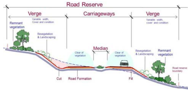
Fig. 2 Typical primary highway section
