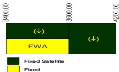
Fig. 1 Malaysian spectrum plane for 3400-4200MHz
