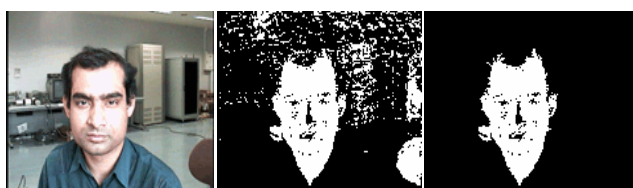
(a) Original image (b) Skin color segmented (c) Face area detected Fig. 4 Skin color segmentation
