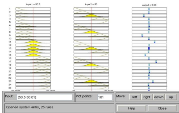
Fig. 10 ANFIS Rule base of Water bath system
