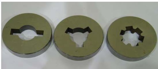
Fig. 6. Toothed dies cavity (2-3-6)
