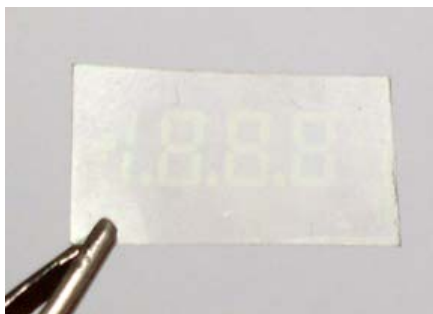
Fig. 5 Photo of the real structure, patterned by photolithographical process on the polymer sheet
