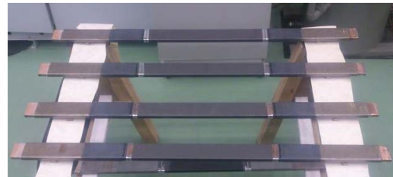
Fig. 7 Setup of sample to measure the tangent delta
