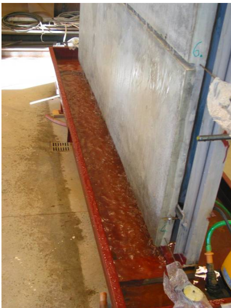
Fig. 6 Sprinkling glass-fiber-concrete façade panel: view to water simulating rain effects
