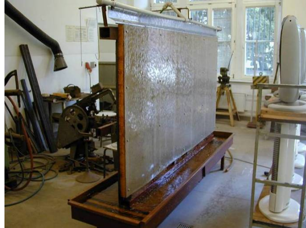
Fig. 17 Sprinkling fiber-cement slabs: view to water simulating rain effects
