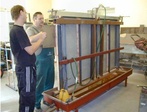
Fig. 14 Installation of test specimen and test equipment for warming and sprinkling fiber-cement slab
