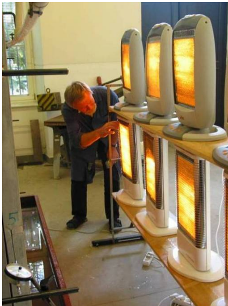
Fig. 15 Warming fiber-cement slab: preparation of equipment
