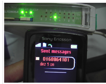
Fig. 5 Receiving text message to trigger digital output
