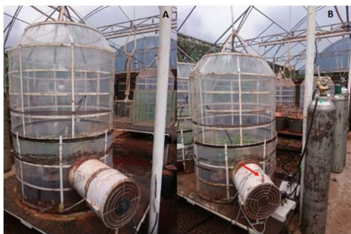
Fig. 1 OTCs used in the experiments. Control without CO 2 injection (A), enriched treatment with CO 2 (B)
