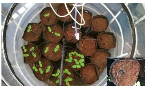
Fig. 2 Irrigation system in the OTCs' vases
