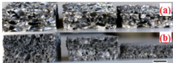
Fig. 8 15%, 25% and 45% deformed sample (start from left to right): (a) HD (bottom) and (b) LD (top)
