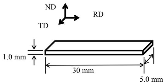
Fig. 1 Dimensions and directions of bending specimen
