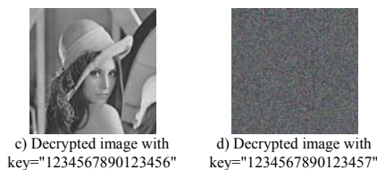
Fig. 8 Key sensitive test result 3 with RC5-32/16/16
