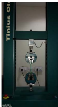
Fig. 2 Experimental setup for tensile testing
