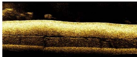
Fig. 8 2-MHz Sonar data after correction
