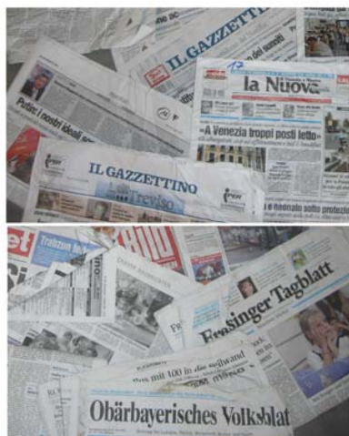
Fig. 1. Visually flexo-printed newspapers (top) and offset-printed newspapers (bottom) are hardly distinguishable. Even experts can identify flexo-printed only by the newspaper title (e.g. Daily Mail, Il Gazzettino) or a magnifying glass. NIR spectral imaging identifies flexo-printed newspapers in real-time and thus enables the development of industrial sorting systems.
