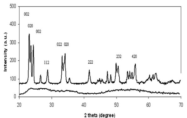
Fig.3 XRD patterns of amorphous (a) and crystallized (b) WO<sub>3</sub> thin films
