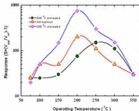
Fig.6 the response of pure and catalyzed films of WO<sub>3</sub> in Hydrogen concentration 0.1% versus operating temperatures
