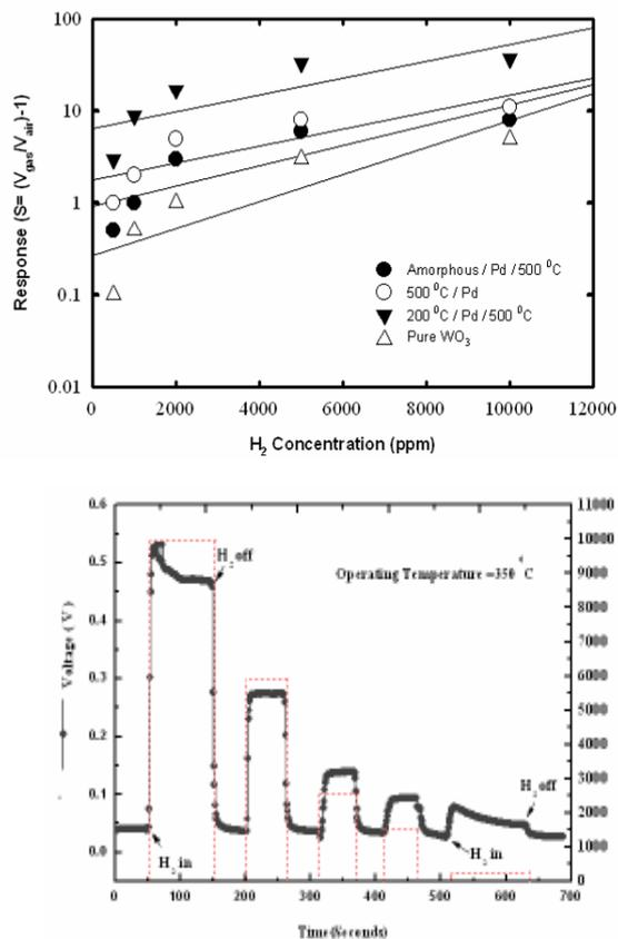
Fig.5 Response of pure and catalyzed films to different Hydrogen concentrations for samples at 350 °C (a) and a typical variation in electrical conductivity versus time for annealed film at 200 °C (b)
