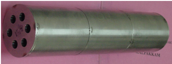
Fig. 11 Orifice assembly for blanket zone (Typical)
