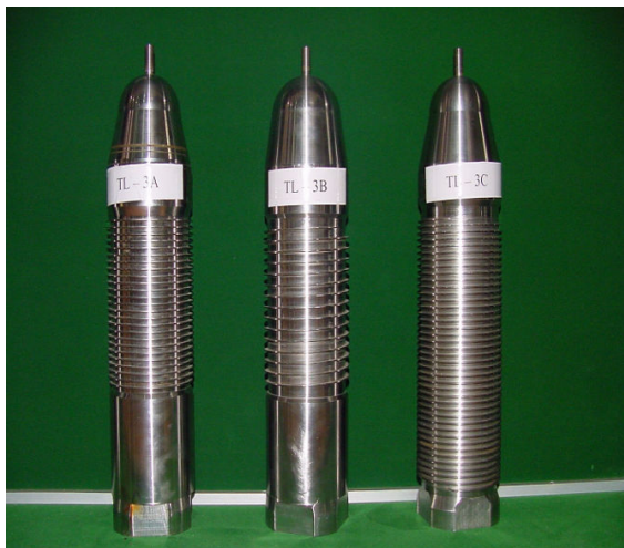
Fig. 15 Top labyrinths for model testing
