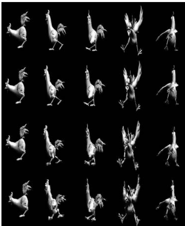
Fig. 11 A selected set of reconstructed Chicken Crossing animation using the hybrid approach. The top row is the original one. The reconstructed animation by using Max Distance threshold = 5%, 10% and 15% are shown in row 2, 3, and 4 respectively. The compression ratio is 47:1, 77:1 and 112:1 in row 2, 3 and 4 respectively.
