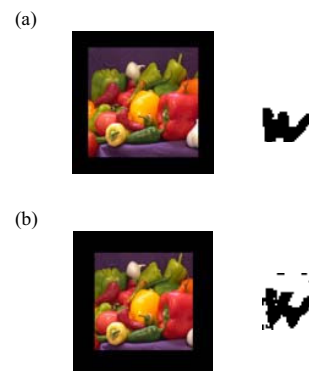
Fig.6 (a) Watermarked image cropped by 226×226 mask along with its extracted watermark, (b) Watermarked image cropped by 216×216 mask along with its extracted watermark
