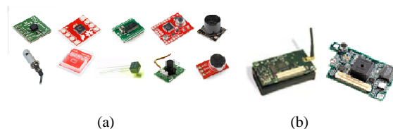
Fig. 1 (a) Ten different sensor modules; (b) MicaZ wireless module and a sensor board
