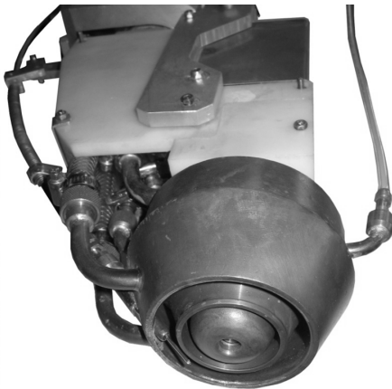
Fig. 3 Plasmatron of APS – 01 machine
