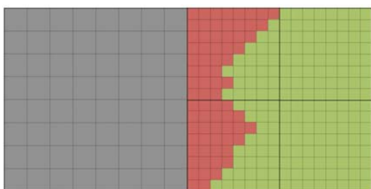
Fig. 8 Representation of the border zone between a high-resolution (HR) dataset (green, on the right) and a low-resolution (LR) one (grey + red, on the left). The tile on the left covers only LR data and do not need further splitting while the presence of HR data on the right one require an additional pyramid level. In the red zone the LR data is oversampled at the resolution of the HR data (not available in this portion)
