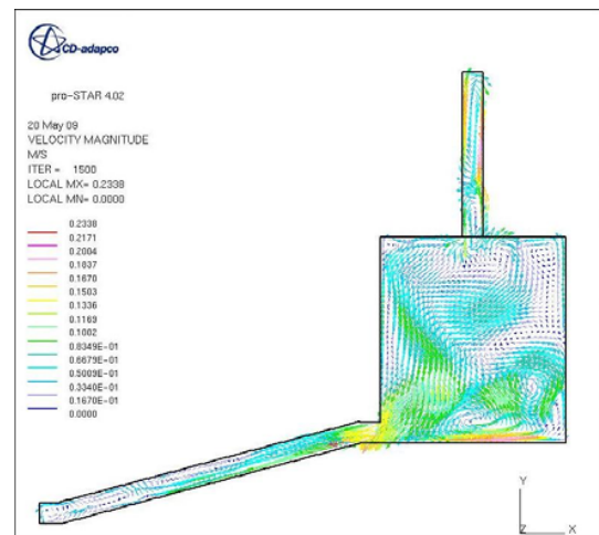
Fig. 3 Velocity distributions for natural convection
