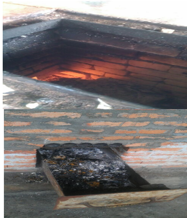
Fig. 4 Inside view of the Incinerator and ash produce after incineration
