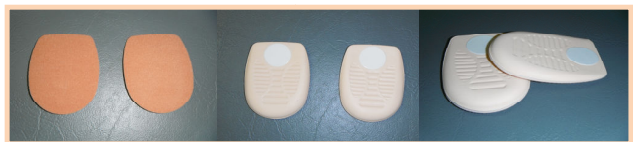
Fig. 8 Specimen 2 (natural latex foam)
