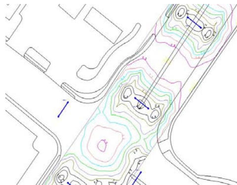
Fig. 2 An example of iso-illuminance contours of an intersection using an imported map from GIS.
