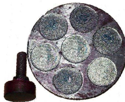
Fig. 3. Copper Electrode and AISI D2 workpiece
