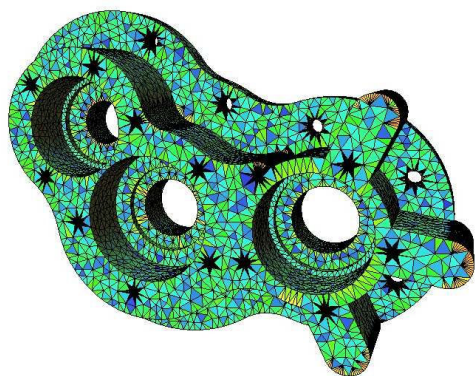
Fig. 9. Pump carter [13]. Colormap according to quality of triangles.
