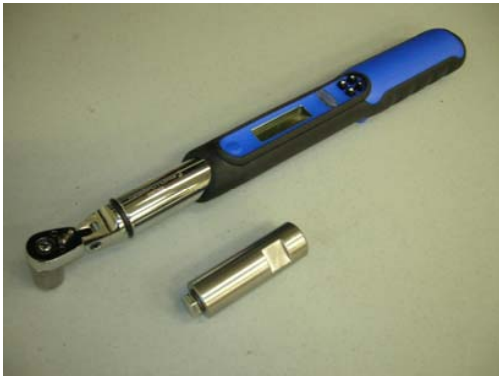
Fig. 8 Torque Wrench and Adapter Tool
