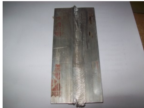
Fig. 11 Friction stir welded aluminum alloy H20 triangular tool
