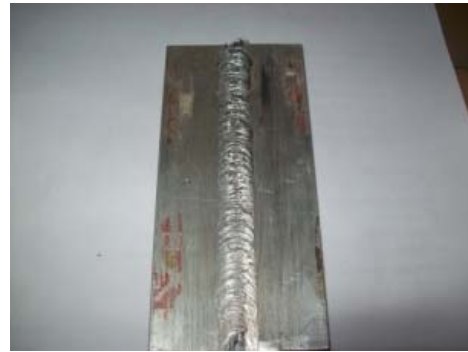
Fig. 13 Friction stir welded aluminum alloy H20 straight cylindrical tool
