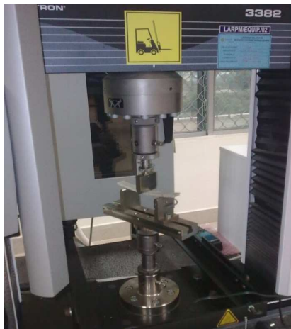
Fig. 5 Experimental setup for ENF Test
