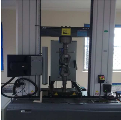
Fig. 4 Experimental set up for DCB Test
