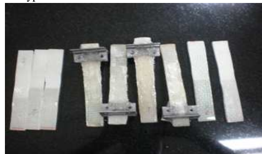
Fig. 3 Specimens for both DCB Test and ENF Test
