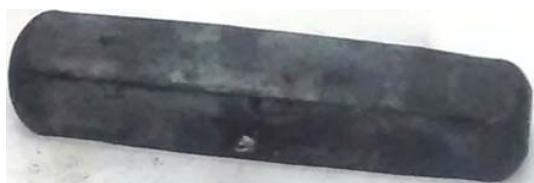
Fig. 3 Sample after 50% diameter reduction
