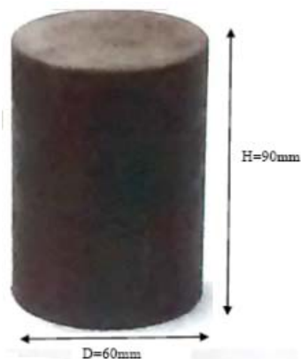
Fig. 2 Sample prepared; D= 60 & H= 90 mm
