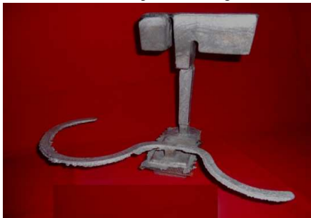
Fig. 4 Double spiral casting of A713 alloy with gating system
