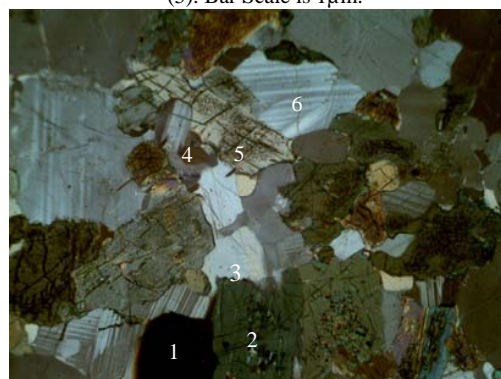
Fig. 7: Photomicrograph of Charnockite (Ak007b a) showing hornblende (1), biotite (2), quartz (3), zircon (4), hypersthene (5) and plagioclase (6). Bar Scale is 2µm.
