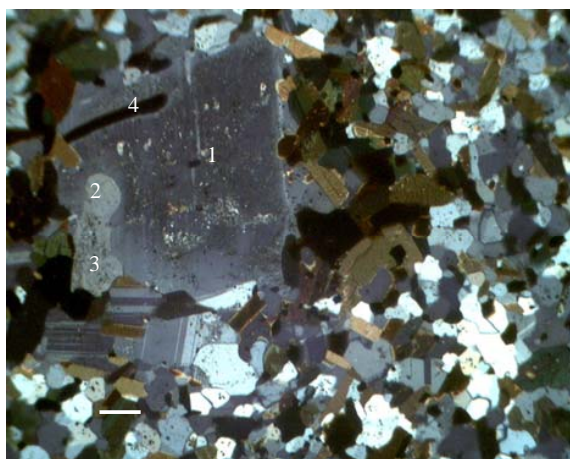
Fig. 9: Photomicrograph of Hybrid rock (H2 b) showing plagioclase xenocryst (1), inherited quartz (2), inherited feldspar (3) and biotite intergrowth (4). Bar Scale is 1 \mu m.
