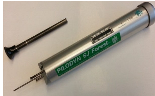
Fig. 1 Pilodyn 6J indentation device
