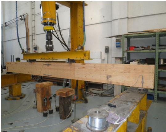
Fig. 4 Four point bending test
