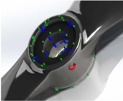
Fig. 4 An example of simulated Gemfan 1147 propeller fixtures
