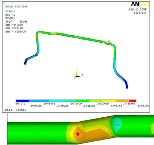
Fig. 7 The effective stresses, based on the greatest stress amplitude of the time history illustrated in Fig. 5
