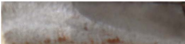
Fig. 2 Quarter elliptical shape of crack observed
