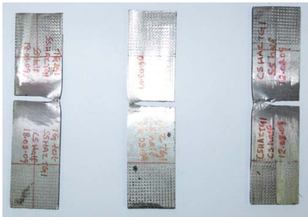
Fig. 1 FCG tested welded specimens
