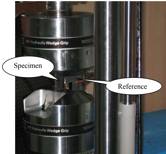
Fig. 3 Specimen mounting details for IRT test
