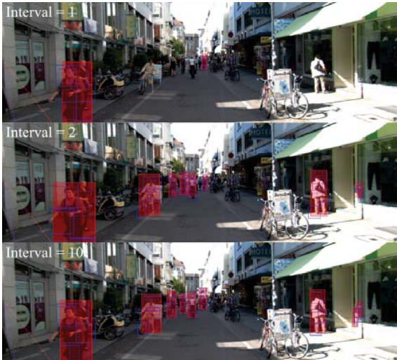
Fig. 14 Detections using interval=1,2,10. Increasing interval from 2 to 10 does not lead to any additional detection
