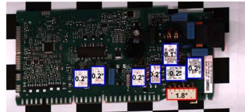
(b) Inspection results for a defected board
