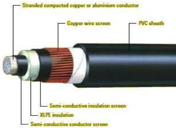
Fig. 17 Cross-sectional area for the 11KV cable
