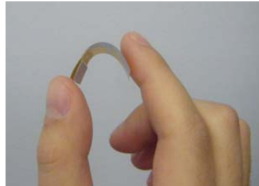
Fig. 1 Wearable inkjet-printed monopole antenna based on a Kapton Polyimide platform
