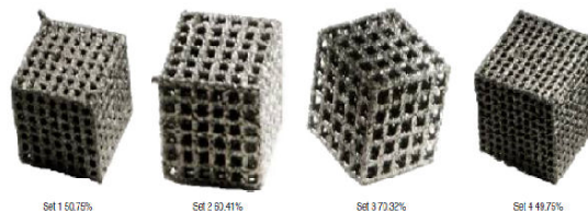
Fig. 11 Different porosities of Ti6Al4V parts fabricated with the EBM system [97].
